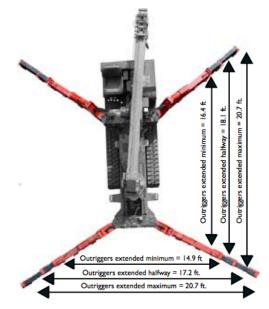
LOAD CHART Lifting capacity varies depending on outrigger configuration and boom length and angle.
